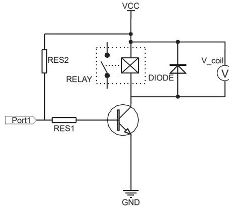
3) In case 5V of transistor drive circuit, it is recommended to use 4.5V type relay, and 3V to use 2.4V type relay.
