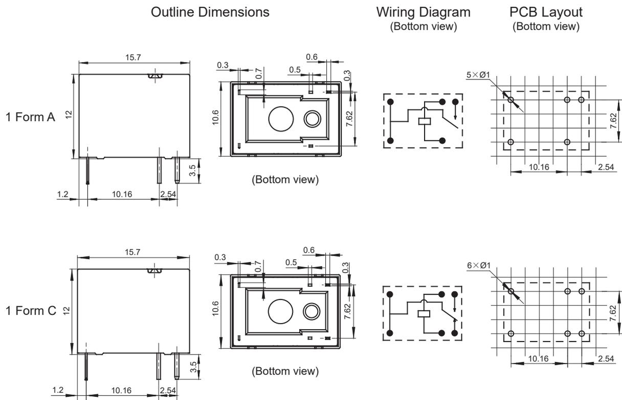
Remark: 1) The pin dimension of the product outline drawing is the size before tinning(it will become larger after tinning),and the mounting hole size is the recommended design size of the PCB board hole.The specific PCB board hole design size can be mapped and adjusted according to the actual product.
