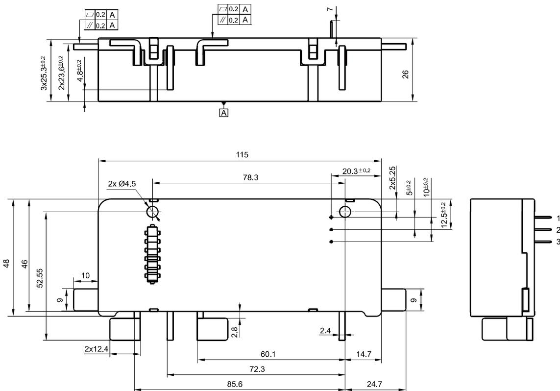
Remark: In case of no tolerance shown in outline dimension: outline dimension  $\leq 1$ mm, tolerance should be  $\pm 0.1$ mm; outline dimension  $> 1$ mm and  $\leq 5$ mm, tolerance should be  $\pm 0.2$ mm; outline dimension  $> 5$ mm, tolerance should be  $\pm 0.4$ mm.
