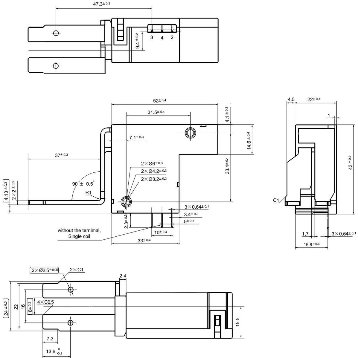
Remark: In case of no tolerance shown in outline dimension: outline dimension  $\leq 1$ mm, tolerance should be  $\pm 0.1$ mm; outline dimension  $> 1$ mm and  $\leq 5$ mm, tolerance should be  $\pm 0.2$ mm; outline dimension  $> 5$ mm, tolerance should be  $\pm 0.4$ mm.
