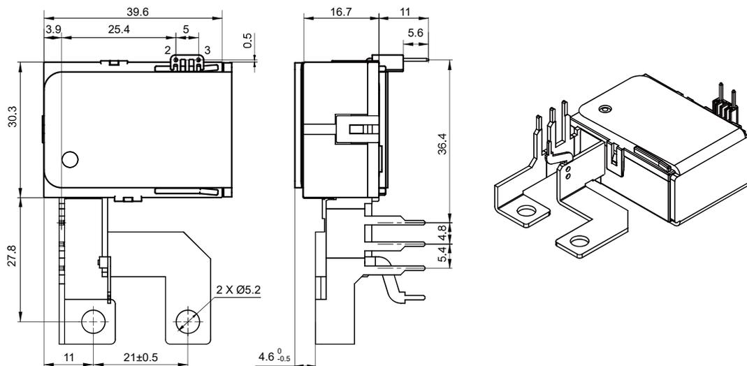
Note: 1) In case of no tolerance shown in outline dimension: outline dimension  $\leq 1\text{mm}$ , tolerance should be  $\pm 0.2\text{mm}$ ; outline dimension  $> 1\text{mm}$  and  $\leq 10\text{mm}$ , tolerance should be  $\pm 0.3\text{mm}$ ; outline dimension  $> 10\text{mm}$ , tolerance should be  $\pm 0.4\text{mm}$ .
