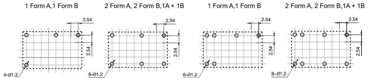
**Remark:** 1) In case of no tolerance shown in outline dimension: outline dimension  $\leq 1\text{mm}$ , tolerance should be  $\pm 0.2\text{mm}$ ; outline dimension  $> 1\text{mm}$  and  $\leq 5\text{mm}$ , tolerance should be  $\pm 0.3\text{mm}$ ; outline dimension  $> 5\text{mm}$ , tolerance should be  $\pm 0.4\text{mm}$ .
