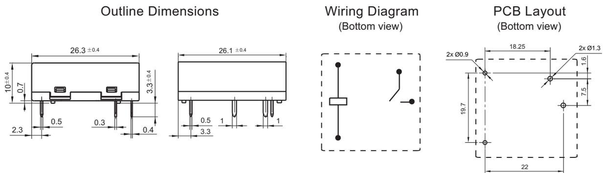
Remark: 1) In case of no tolerance shown in outline dimension: outline dimension  $\leq 1$ mm, tolerance should be  $\pm 0.2$ mm; outline dimension  $> 1$ mm and  $\leq 5$ mm, tolerance should be  $\pm 0.3$ mm; outline dimension  $> 5$ mm, tolerance should be  $\pm 0.4$ mm.
