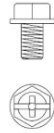
C type on 25-40A FLA #10-32 combination Phillips, slotted & 5/16 hex head with #8 washer
